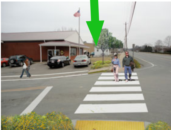
Above: The intersection of South Main Street and Hunsucker Street at the post office. Adding a high-visibility marked crosswalk, advanced stop line, and better defined curb ramps would enhance this crossing for pedestrians.
