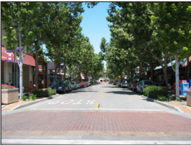
Brick or cobblestone streets help slow traffic and create a feeling that the street is not a highway or fast-moving arterial.
