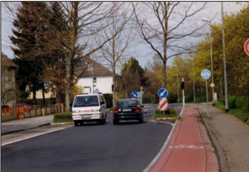
The choker produces a narrow passage for vehicular traffic.
