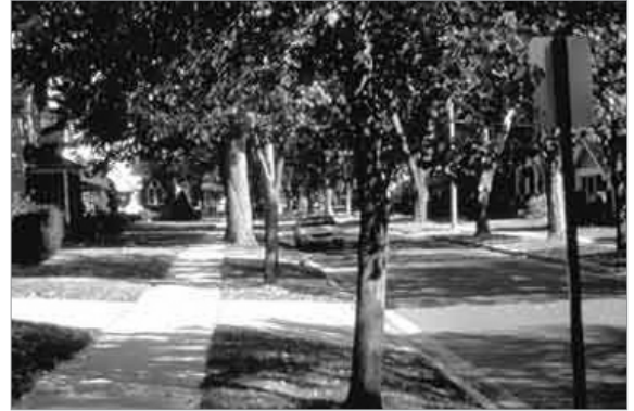
A well designed residential sidewalk will have a width of at least five feet. (Image from http://www.walkinginfo.org )
